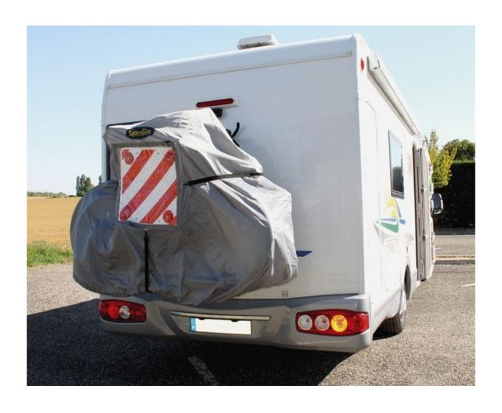
The V-20 sign is made of aluminium but other durable materials are acceptable
