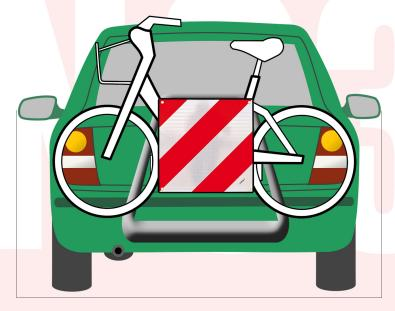
You must display the V-20 sign located at the END of the load and perpendicular to the axis of the vehicle
