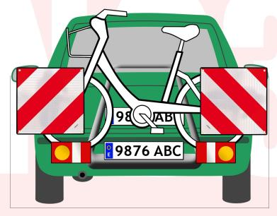
If the number plate OR lights are hidden by the load, an additional lighting and signalling device, plus an additional number plate, must be placed to the rear of the load
