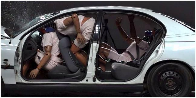
In these other images we can see how the passenger at the rear hits the driver of the vehicle with their head, in turn displacing the front seat with their weight, producing injuries to the driver in the head and knee that could have been avoided.
